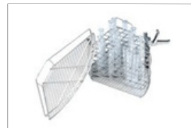
E 149 insert 1/4, for 80 test tubes up to 16 x 105 mm, 80 compartments. Mesh width on the base 8 x 8 mm
