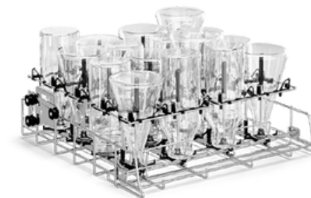
C1834 with two docking connections for up to 2 injector modules or inserts. Automatic closing of the connections when not in use. For use on all levels. Loading surface: W 507 mm, D 520 mm
