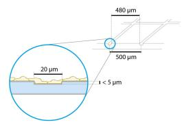
The grooves are 20  $\mu$ m ( $\pm$  5  $\mu$ m) wide and approximately 5  $\mu$ m deep. Cells can grow in the grooves as well. We recommend using objective lenses up to 20×. Anyhow, the optical quality meets the requirements of 63× and 100× oil objective lenses as well (glass coverslip bottom, No. 1.5H).
