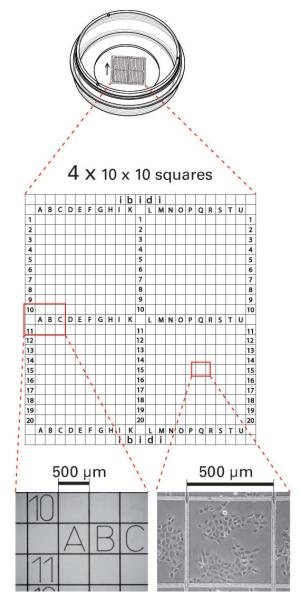
Microscopic images of the grid. Left: 4x objective lens brightfield without cells. Right: 10x objective lens phase contrast with rat fibroblast cells.
