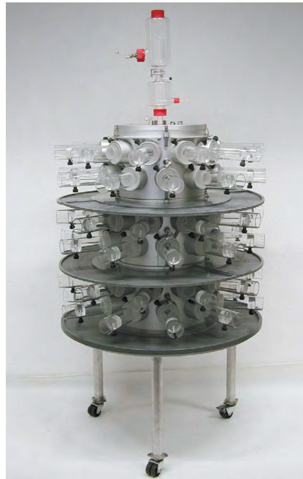
Head Nose Only Unit with aerosol conditioning units
