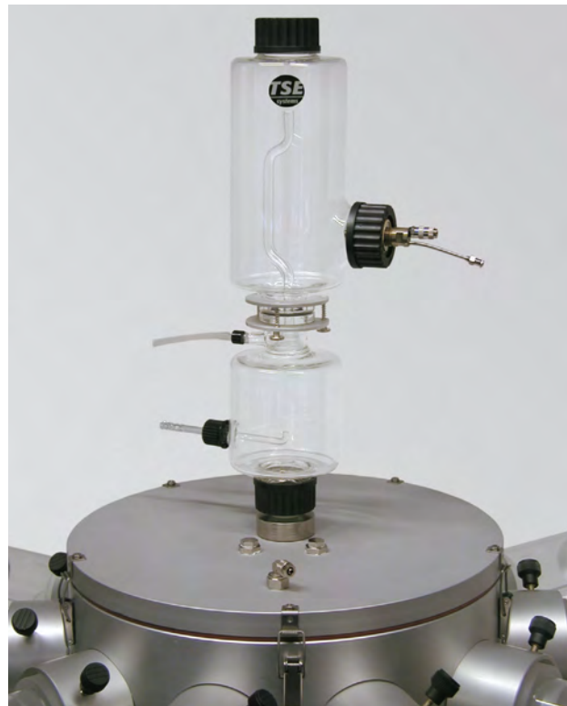
Aerosol nozzle – mounted on preseparator
