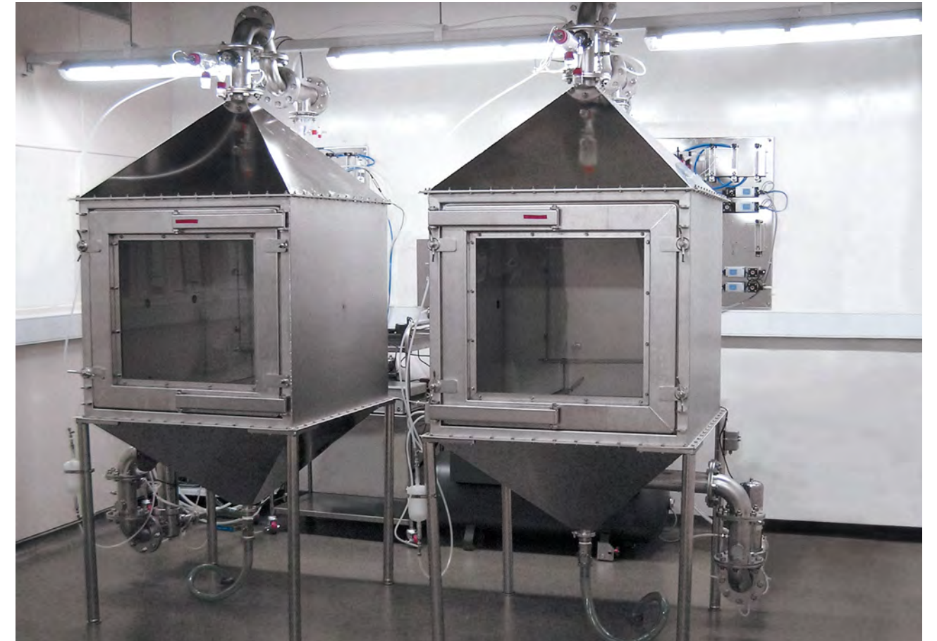
Whole Body Units with aerosol conditioning and exhaust air line – in the background a mounting panel with flow control units
