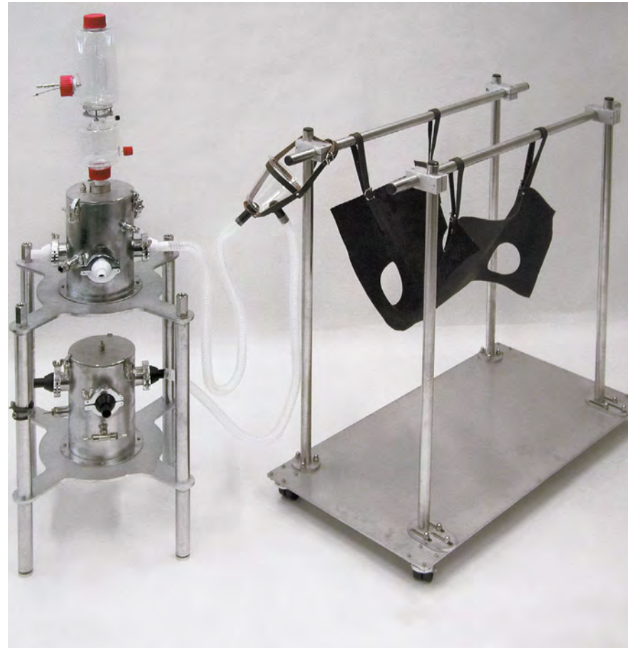
A Dog Exposure Unit for the application of liquid aerosols with inhalation mask, holding device and leather harness for the dog
