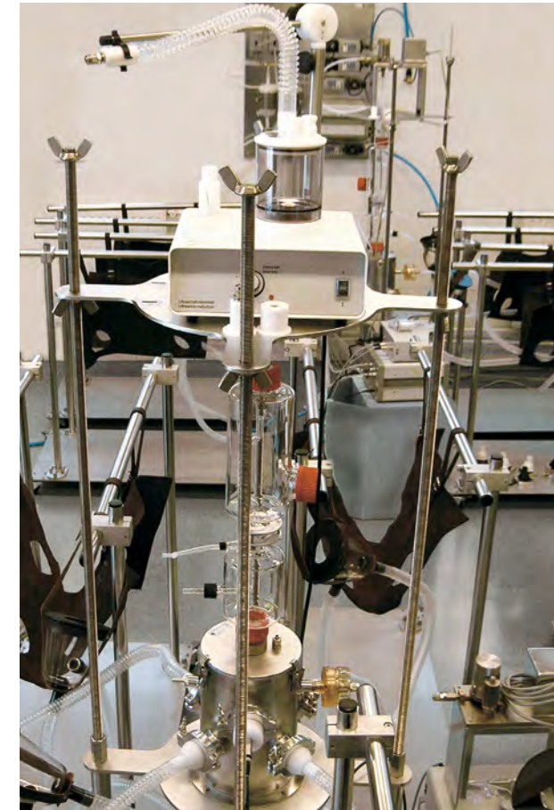
Dog Exposure Unit with ultrasonic nebulizer
