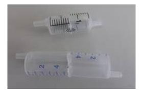
Figure 4 Example of a simple DIY bubble trap.
